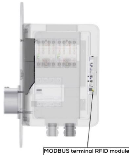
Figure 3 Modbus cable connection
