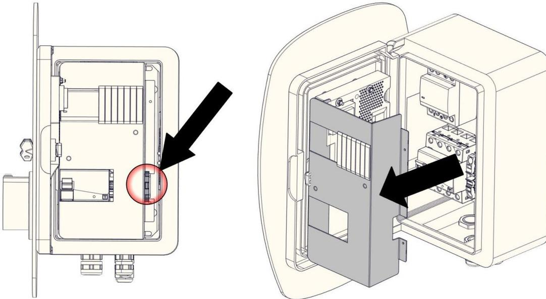
(1) Install the PNI on the free top-hat rail in the upper right corner.
