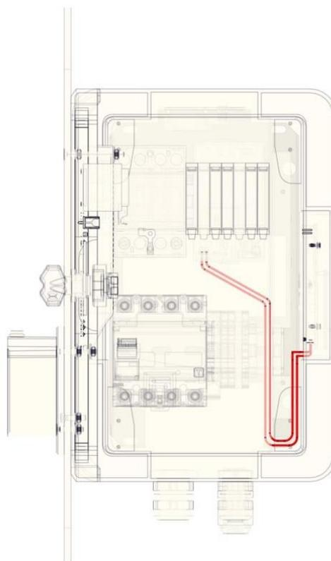
Figure 4 Recommendation Modbus cable routing
